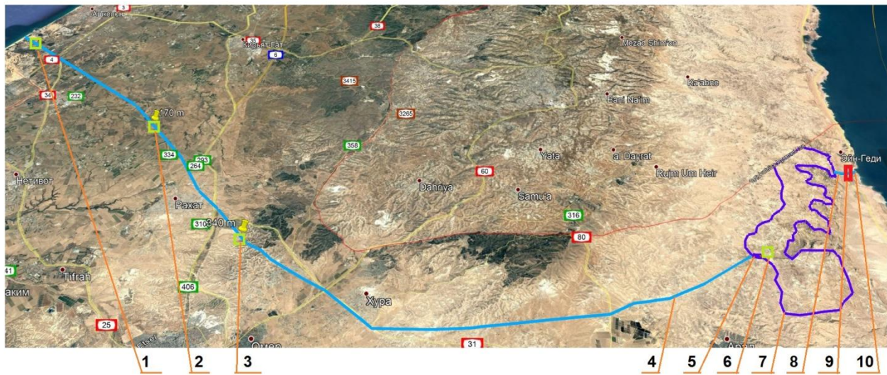
1- 1st pumping station, 2- 2nd pumping station, 3- 3rd pump station, 4- conduit 88.5 km, 5- 0.13 km 2 reservoir, 6- 4th pump station, 7- blue contour 77 km 2 , 8- conduit 1.6 km, 9- water-power plant, 10- open channel
